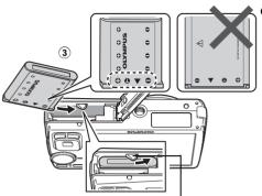
Insert the battery by putting in the ▼ marked side first, with the ⊕ marks toward the end of the camera, the ⊕ marks toward the center of the camera.
